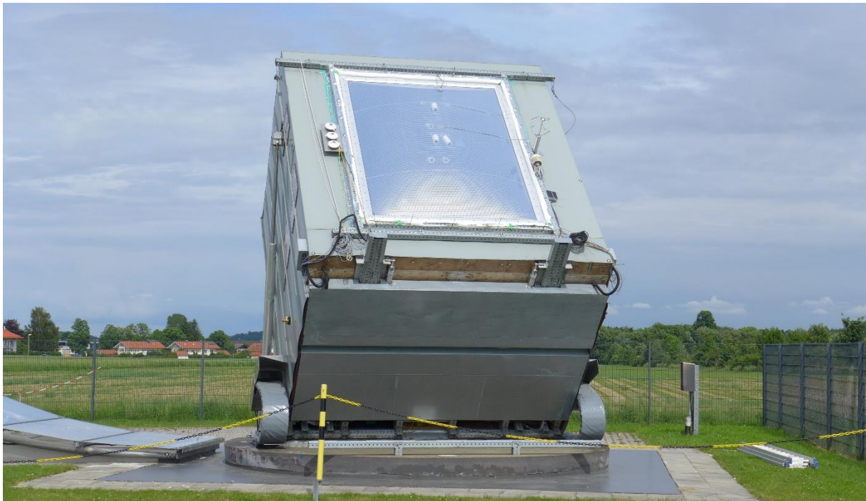
Figure 4.1: Calorimetric Façade and Rooftop Test Facility with the "MEM1" specimen.
